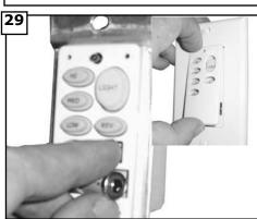
Remove cover by snaping off from top or bottom. Install 12V battery into wall remote. Duracell MN21 / Eveready A23 / GP 23A all 12V.
